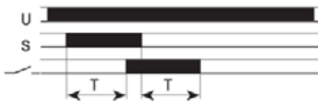
FZ16: ON Delay (1 timed contact + 1 instantaneous contact)
