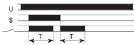
FZ12: Signal ON and OFF delay
